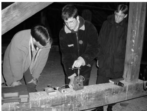
Figure 1 – Laboratory sessions. Students are testing a roof structure by a screw withdrawal resistance meter and evaluate a plane tree by an acoustic tomograph in winter.
