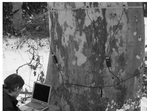
Figure 1 – Laboratory sessions. Students are testing a roof structure by a screw withdrawal resistance meter and evaluate a plane tree by an acoustic tomograph in winter.
