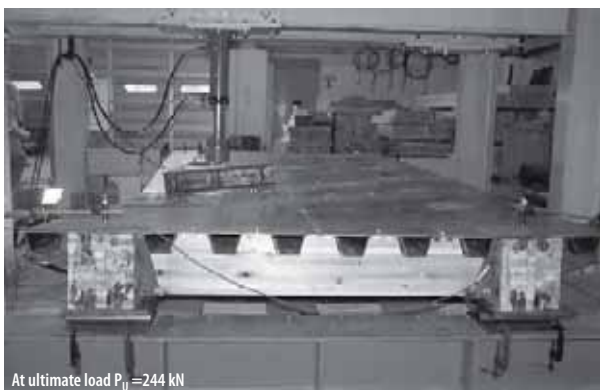
Fig. 9 Bridge model shown during loading
