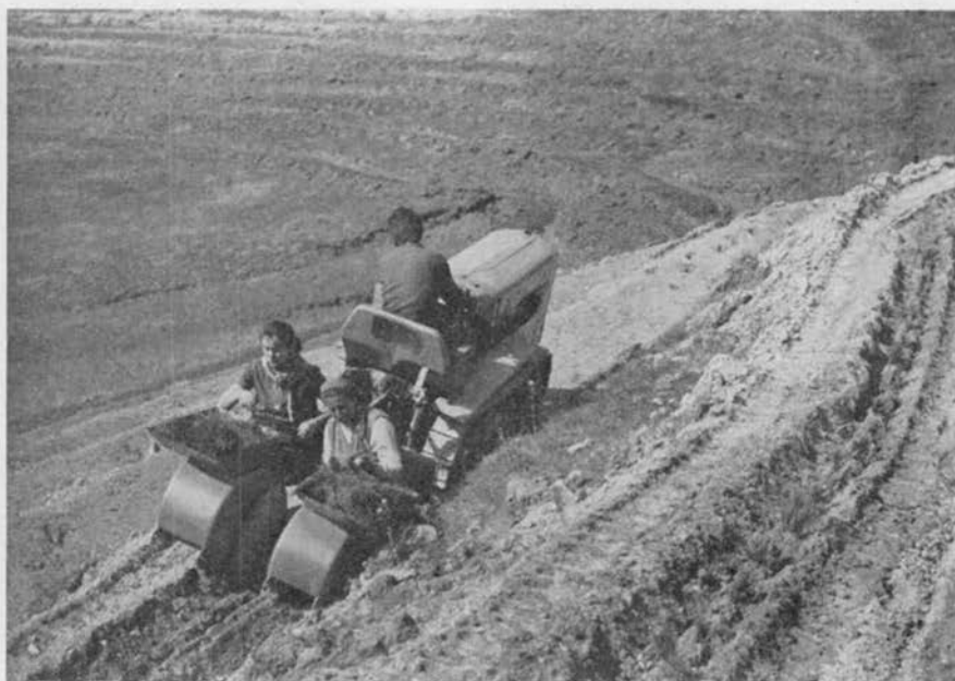
Figure 3. Plantation with FPÜ-1-type single-row planter (Developed by ERTI) (Photo: M. Adamik)
