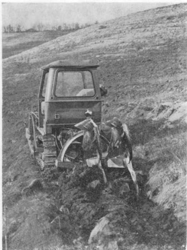
Figure 2. FPVE-2 tractor plough (Developed by ERTI) on TL-30 type narrow-track Bulgarian caterpillar in action. (Photo: M. Adamik)
